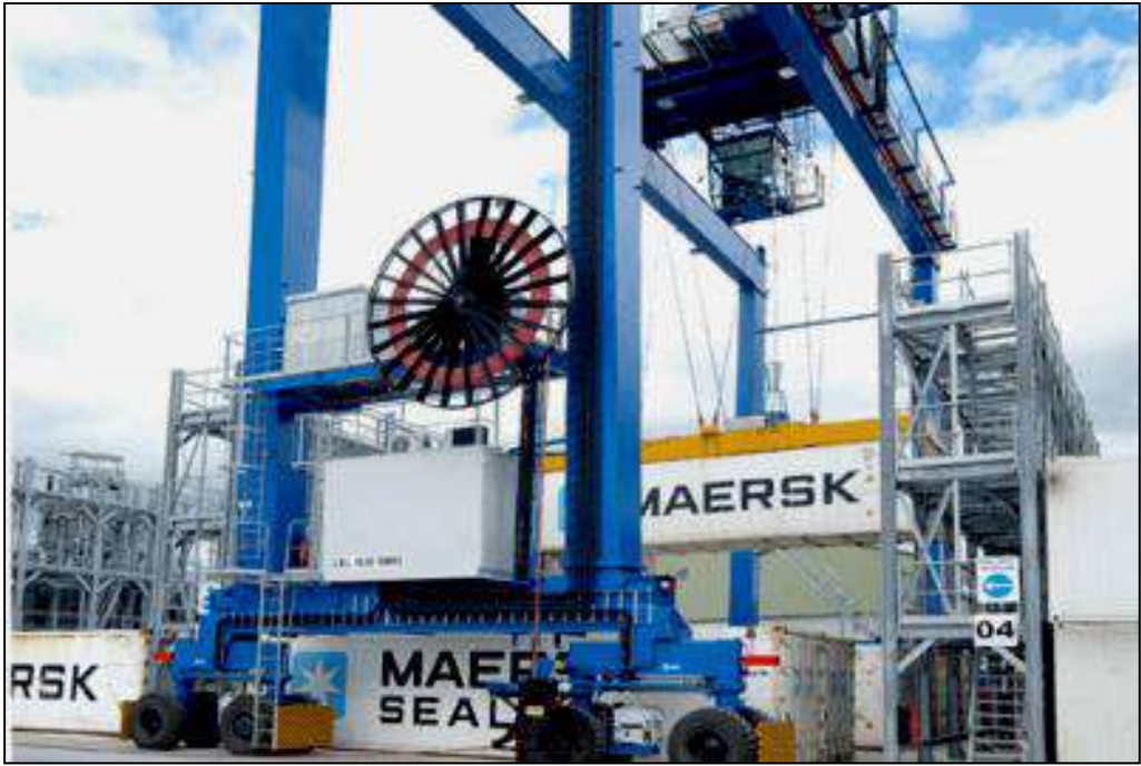
Figure 7.25 Typical E-RTG for Yard Operation
