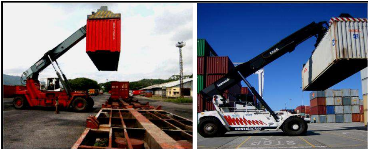
Figure 7.29 Snapshot of Typical Reach Stacker Handling
